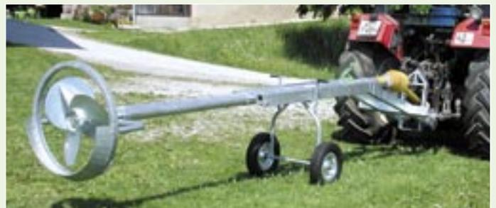
A closed protection ring prevents the mixer blade from being damaged particularly when mixing in narrow and closed pits. In addition, the chopping effect is improved
